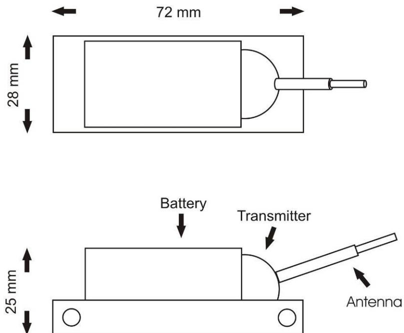
**Fig. 2(b)** H-module SB2 VHF radio transmitter
