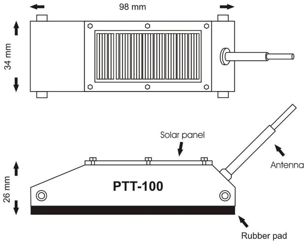
**Fig. 2(a)** PTT-100 GPS/ARGOS transmitter
