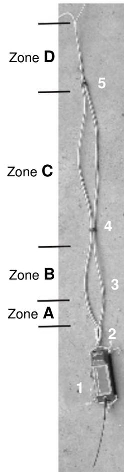
**Fig. 4** Fitting zones for harness for PTT satellite-telemetry and VHF radio-telemetry devices
